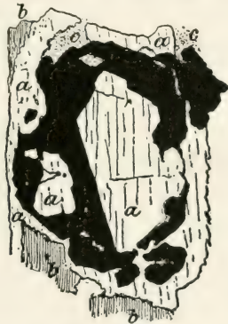
Fig. 7. Primary pyrrhotite in augite. Black, pyrrhotite; a, augite; b, uralite; c, chlorite. From W. Lindgren; 17th Annual Report United States Geological Survey, Part II.
